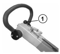
Turn the ignition key (1) from position "1" to position "0". Pull out the ignition key.
